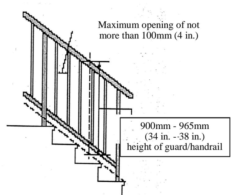
Guardrails are required to be 36 in. minimum
